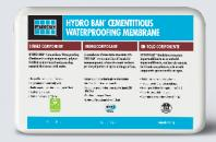
A one component, polymer fortified, cement based waterproofing material that mixes only with water. HYDRO BAN Cementitious Waterproofing Membrane handles negative and positive hydrostatic pressure up to 2 BARS (29 PSI) when applied at 40 mils (1 mm) thick. Flood test within 2 hours.
